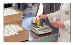
Weighing with tolerance range (checkweighing): a visual signal helps with portioning, dispensing or grading
