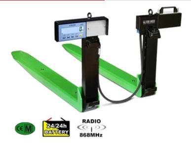
Pair of forks with an integrated weighing system, for lift trucks, easy to use, sturdy, and reliable. Simple and easy to install, these replace the original forks and allow a clear visualisation of the loaded weight. Compatible with any lift truck having a DIN 15173 - FEM fork holder plate, of the IIA (IIB optional) or IIIA class. Available in CE-M approved version.
